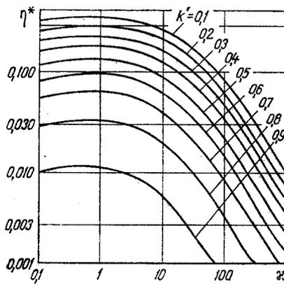
Fig. 2. Dependence of the quantity  $\eta^*$  at the moment of contact of the lower boundary of the bed with the grid on  $\kappa$  with  $v = 0.1$  and different  $k'$ .
