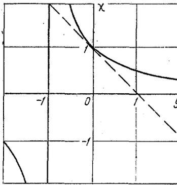
Fig. 4. Coefficients of variation of hydraulic resistance of a bed upon the application of vibrations: solid curve)  $\kappa_p$ ,  $y = \delta q/q_0$ ; dashed curve)  $\kappa_q$ ,  $y = \delta q/\langle q \rangle$ .
